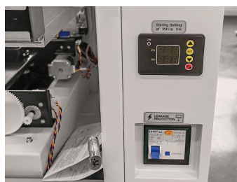
White Ink Stirring Setting & Leakage Device
